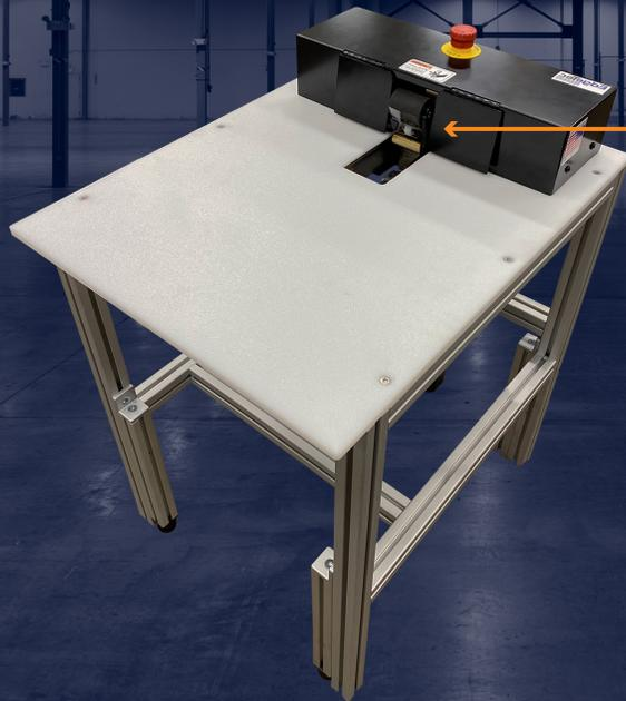
The L-Clip 100 is designed to run tape widths less than 2 inches.
