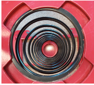
WHITE SPRING IMPROPERLY POSITIONED IN UPPER POCKET
